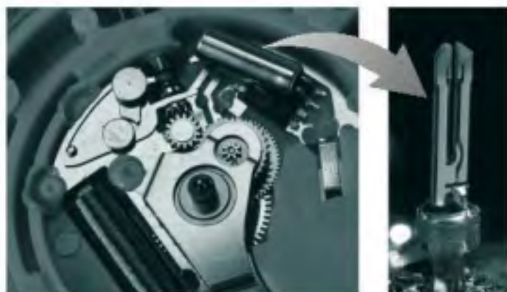
A tiny quartz tuning fork sets the timekeeping of a quartz watch. It oscillates at 32,768 Hz. What does this mean, and why this number?
