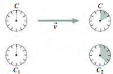
FIGURE 33.7 Clock C moves between clocks C_1 and C_2 , which are at rest relative to each other and synchronized in their rest frame. C measures a shorter elapsed time.
