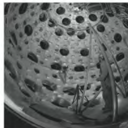
FIGURE 38.20 Target chamber of the National Ignition Facility is 11 m in diameter and weighs 130 tonnes. Holes are ports for the 192 laser beams that converge on the millimeter-sized target.
